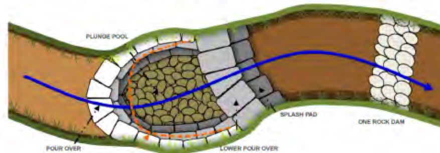
Schematic of Zuni Bowl from Erosion Control Field Guide, Quivira Coalition & Watershed Artisans © 2012 CS AA
