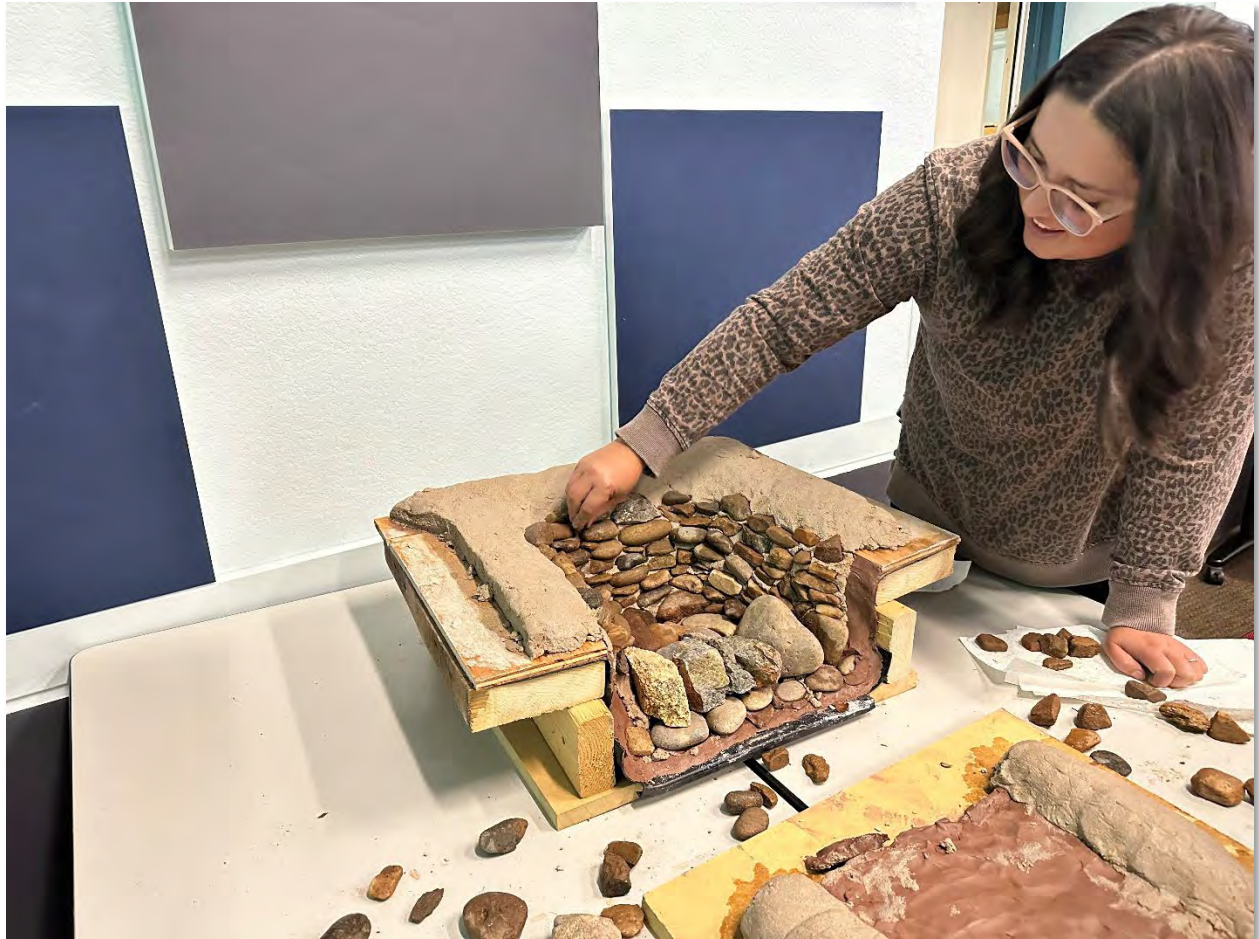
Figure 4-3. NMDOT workshop participant constructing a desktop model of a Zuni Bowl and One Rock Dam.
