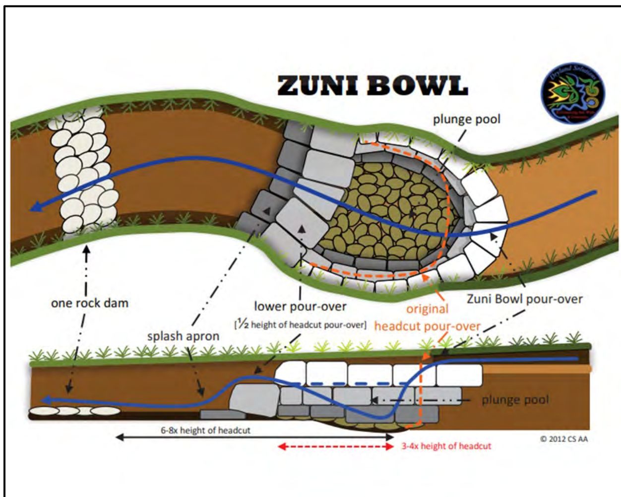
Figure 1-1. Schematic Diagram of a Zuni Bowl (Sponholtz and Anderson 2012).
